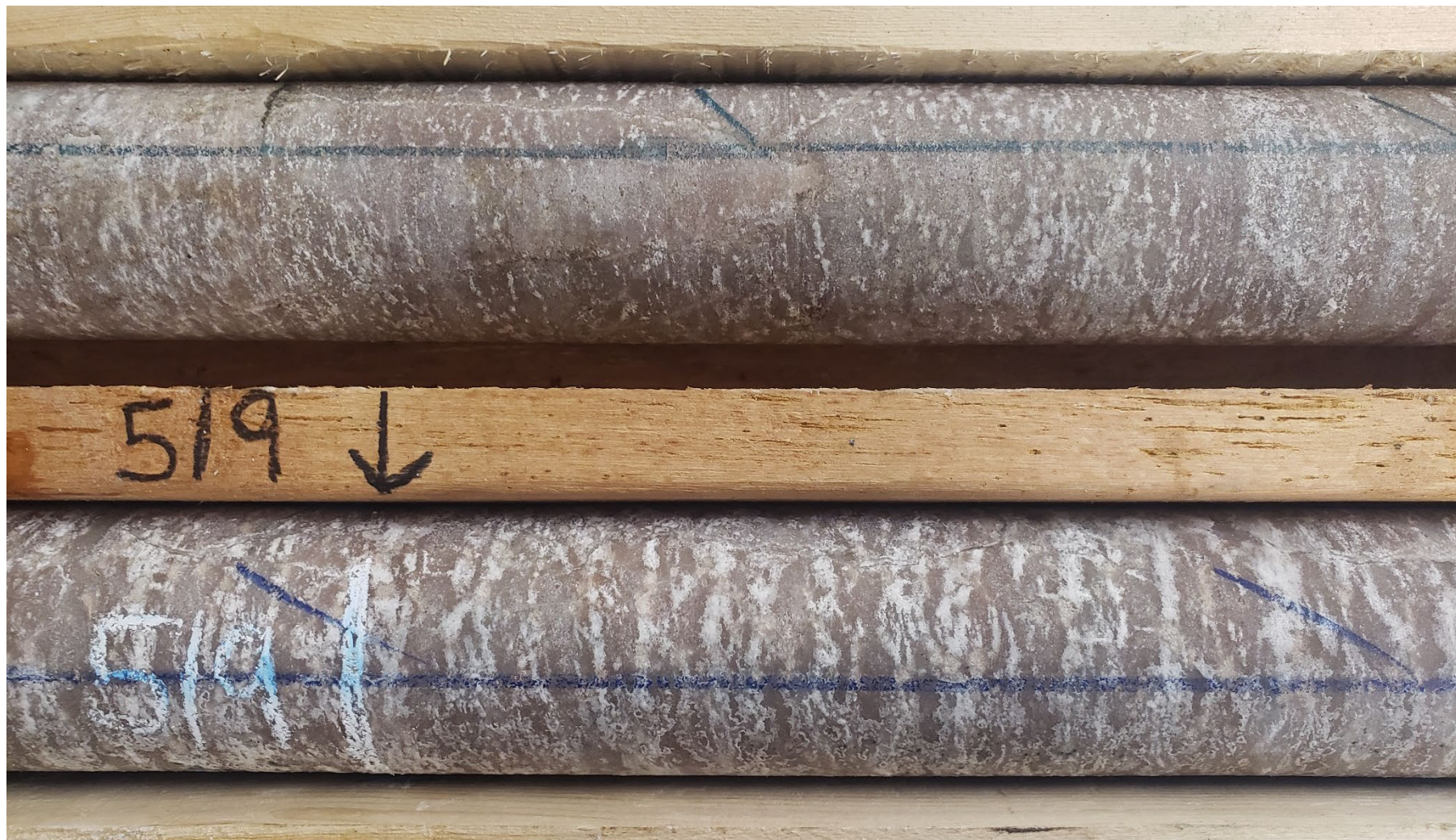
FIGURE 5 – Salt encrusting drill core above and below 519 m in conductive fluid reservoir
