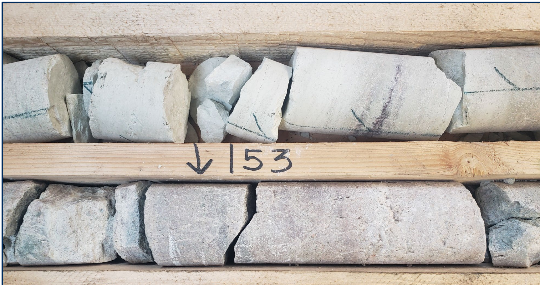
FIGURE 3 – Drill core from conductive fluid reservoir at ~153 m
